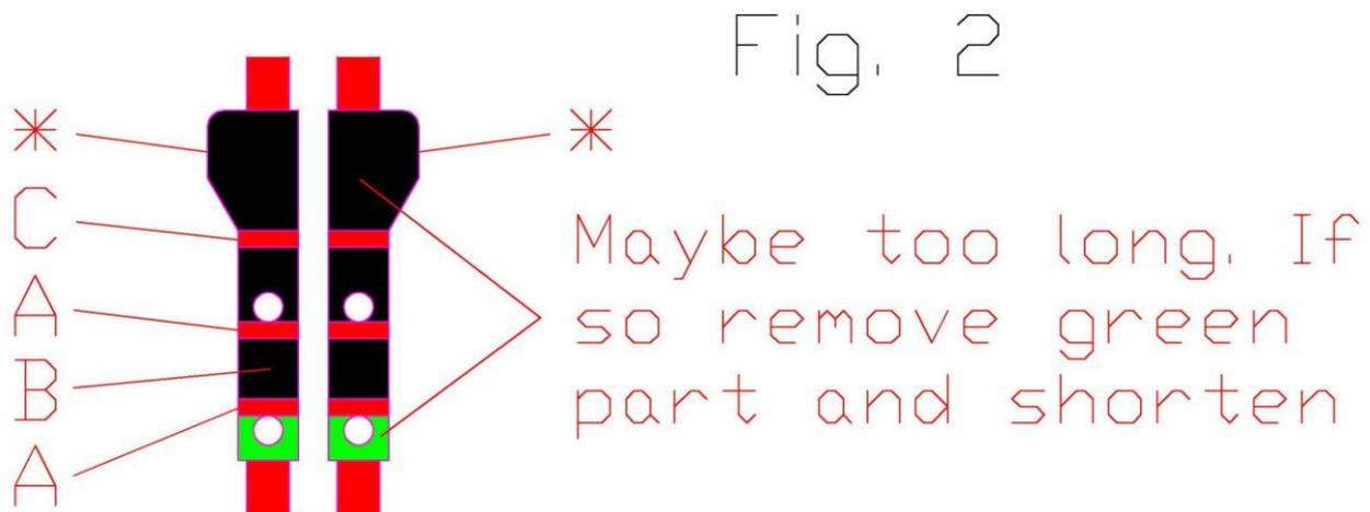
The spring wire will need to be cut so that it is a whisker under 25mm and fits neatly between the insides of the solebars. Thread the wire through the two small holes in the springing mechanism and make sure it is bearing on the vertical part of the buffer retainers. If you want to change the wire for a heavier/lighter gauge simply remove and replace.
