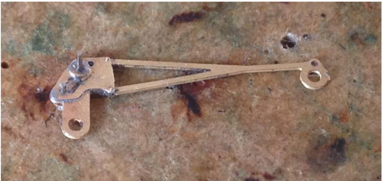
Check that the large holes in the D/C brake ratchet & pawl (8) can accept 0.7mm wire and the small holes 0.3mm wire. These need to be fitted to the brake shaft linkage. Drill a 0.3mm hole in a spare piece of wood and insert a length of 0.31mm wire. Feed the pawl onto the wire as shown in the photo below.
