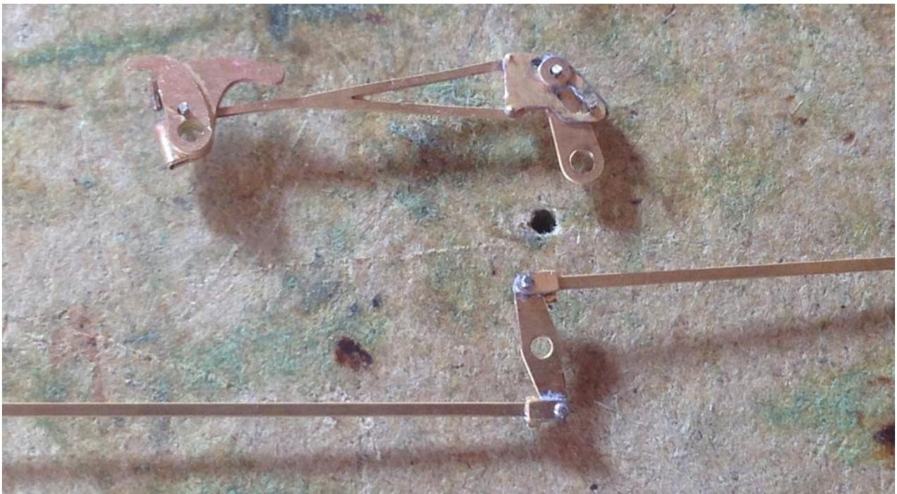
Fit both the brake shaft linkage and bogie linkage to the underframe along with lengths of 0.7mm wire for the brake shafts. Make sure the 0.7mm wire extends 0.5mm or so beyond the vees. The bogie linkage goes along the centre line and the brake shaft linkage goes on the side with the two vees (see photo below).
