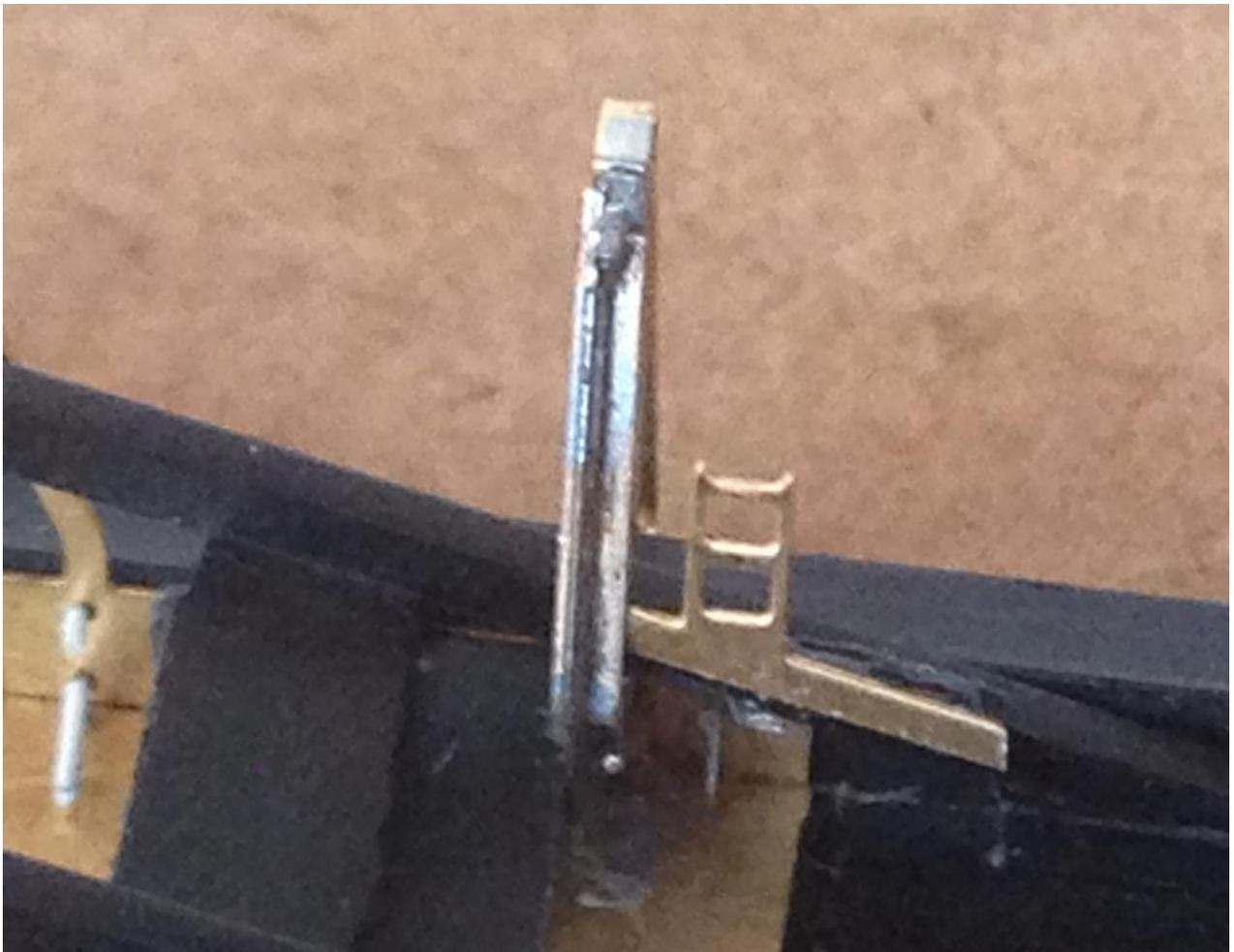
The shunter's pole rack (13) can be removed from the fret and glued in place on the brass angle behind the brake lever guard. Leave about 1mm between the rack itself and the guard/stay.
