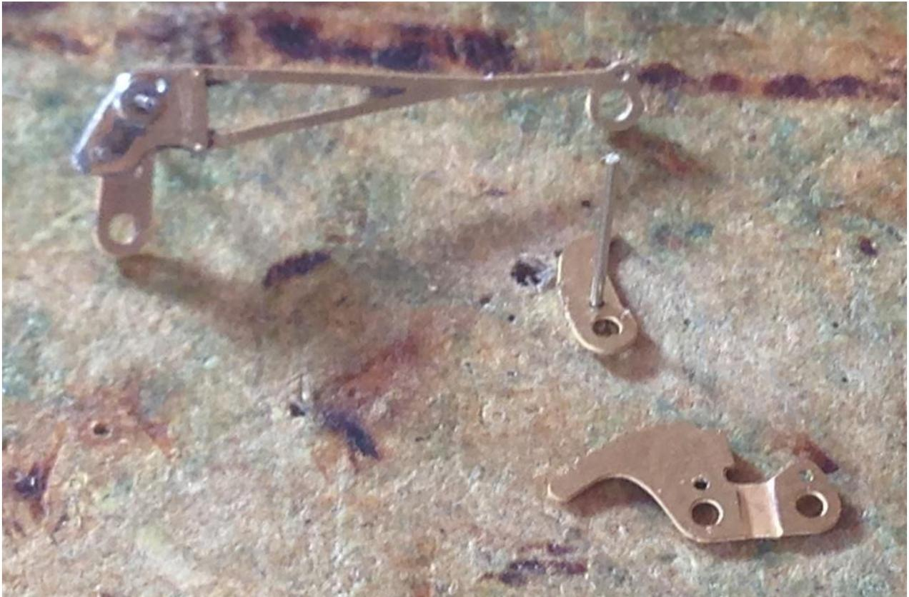
Make sure that the holes in the D/C brake bogie linkage (8) and D/C brake bogie linkage overlays (9) can accept 0.31mm wire and remove from the fret. Attach the overlays by folding around the linkage and then using short lengths of 0.31mm wire to locate them. Solder in place and trim the wire to represent bolt heads. Fold over the locating tab at the end of the linkage.
