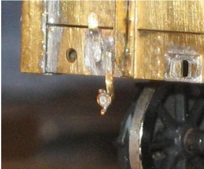
There are D links for fitting to the bolster pins (32). Carefully drill a 0.4mm hole near the base of the bolster pins. The D link can then be gently fitted in place. You will have to prise the sides out slightly to locate them in the holes then close them up again. There are spares in case any go disappearing across the room! Some definitely will...
