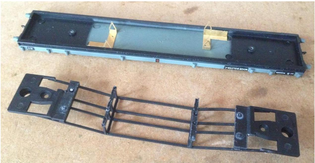
If you are constructing any of the Lever brake options then you will also need to remove a little bit of material from the ends of the trussing where the vees will go. The following photograph will give you a better idea.
