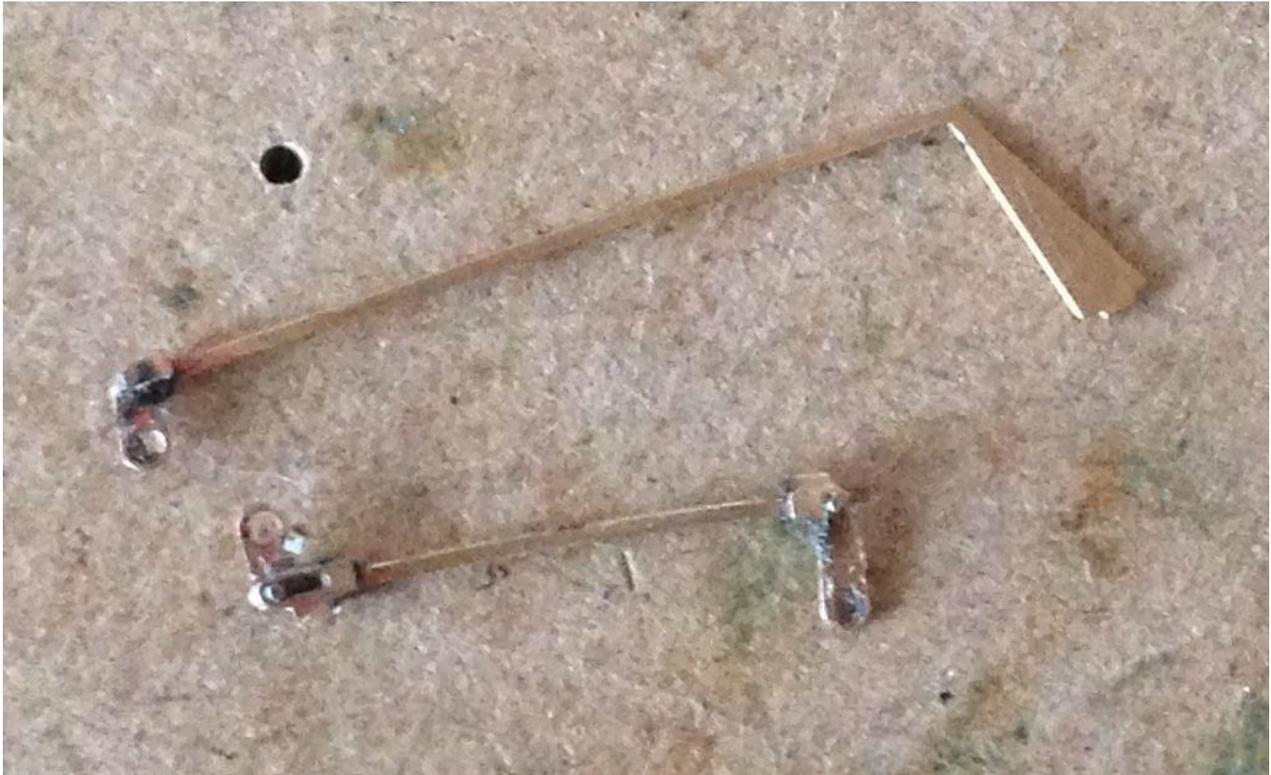
Make sure that the holes in the brake lever actuators (16) can accept 0.8mm wire, remove from the fret and fold out the little clutch. Also make sure that the holes in the vacuum cylinder actuators (22) can accept 0.8mm wire
