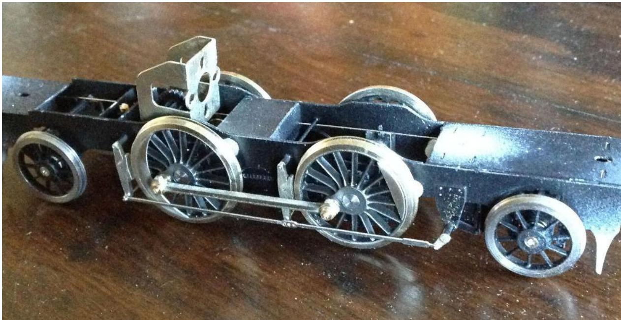
The chassis is designed to be used with High Level hornblocks. These should be attached to the **outside** of the frames. The horncheeks on the High Level hornblocks sit against the top of the cut outs in the main frames.
