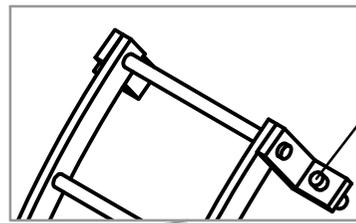
Type A ladder - 0.31mm wire pin for locating on tank
