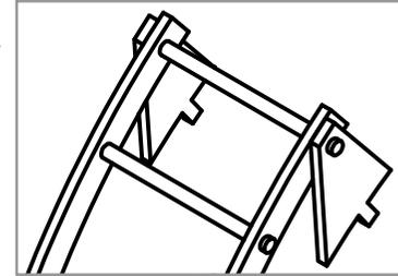
Fold up tops of ladder as per diagram. Wire pin (1) or tab (2) will locate into holes in tank drilled using jig (See page 4).
