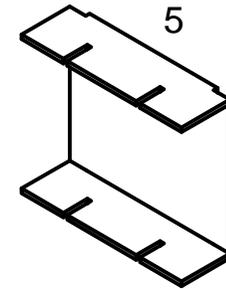
Fold up ladder assembly jig (5) and use to keep sides of ladder aligned.
