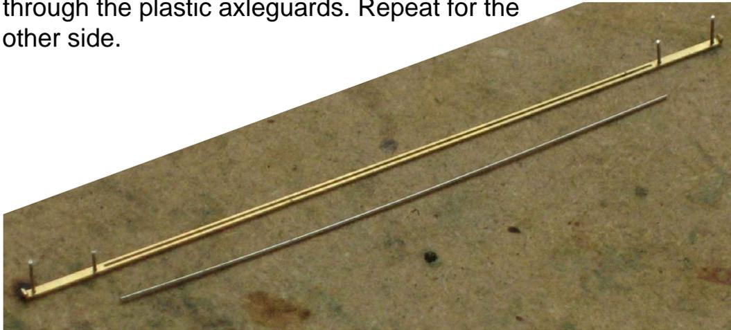
Drill two pairs of 0.3mm holes into a piece of scrap wood. Fold up the end of the tie bar and thread short lengths of 0.31mm wire through the tie bars locating into the holes in the wood. These can then be soldered in place and then filled back to represent bolt heads. You will need to make sure there is at least 0.75mm of wire projecting from the back of the tie bars to locate on the axleguards. Whilst you are at it solder a length of 0.31mm wire into the slot to reinforce the tie bar.
