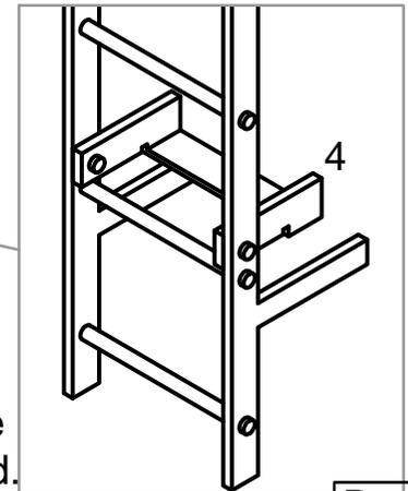
Type B ladder - Prong inserts into hole in Bachmann solebar where plastic ladder was located.
