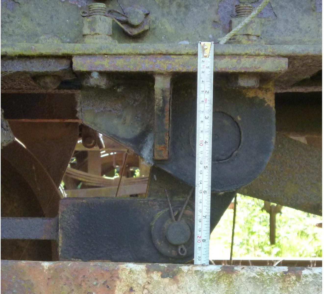
The two vacuum brakegear assemblies can now be fitted to the chassis. Refer again to Fig. 1 for the arrangement. You will need to fit them with a short length of 1.2mm wire for the vacuum cylinder shaft as shown below. Solder the wire to the inner bracket and the vacuum cylinder crank to the shaft at approximately the same position and angle as below. Leave the link free for the moment. Note that the link goes outside of the brakegear and safety loops and inside the axleguard.
