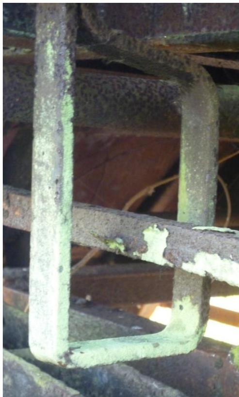
Once the vacuum shaft link and safety loop are in place the main brake cross shaft can be fitted and the rest of the brakegear fitted.
