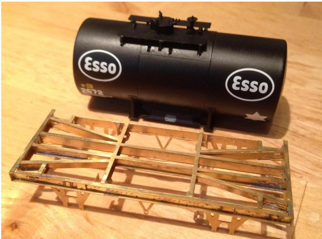
The solebars can now be fitted to the chassis. There are slots and tabs on the bottom plate to aid location and the ends go into the channel that is the headstock. Fit the solebars at an angle and then straighten, locating the slots and tabs at the same time. Once in place then the solebar can be soldered in place.
