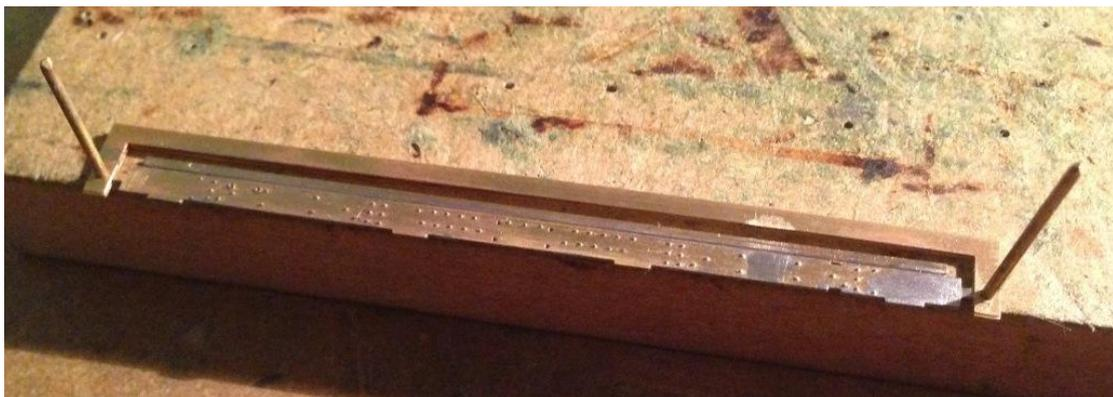
Now is probably the easiest time to attach the solebar detailing to the solebars so I shall cover this now before returning to the business of assembling the chassis.
