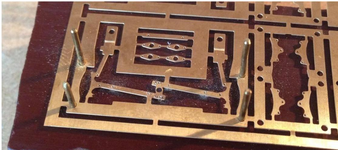
Once the jig is created you can check that the small holes in the rest of the main brakegear (13), brake shoe infill (14), push rod cranks (15) and push rod infills (16) can accept 0.31mm wire. These are marked in yellow on Fig. 3 below. I find it easier to locate the hole from the side with no writing on the main brakegear.
