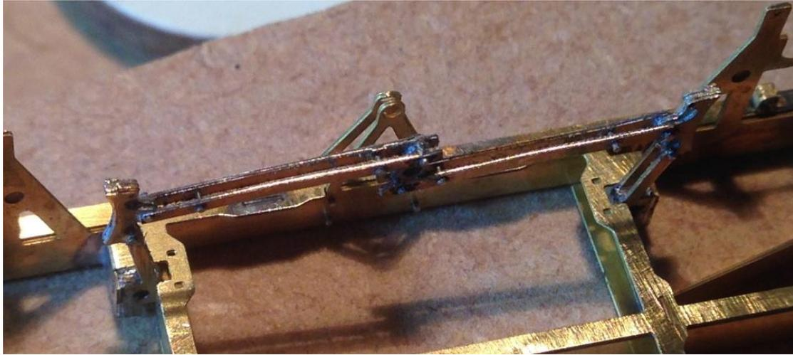
Finally the push rod safety loops (13) can be fitted. These fold up and are soldered in place using very small slots in the bottom plate to align things.
