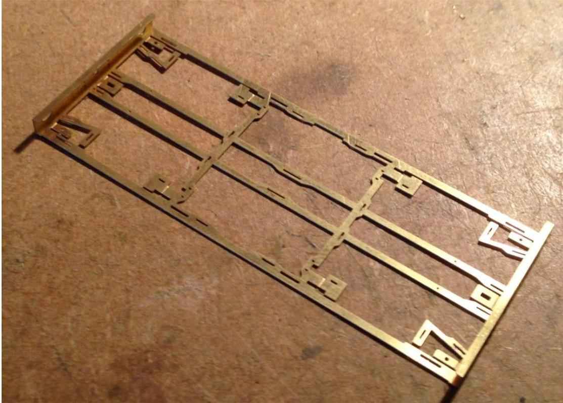
Remove the longitudinal spacers (2) and the transverse spacers (3) from the fret and clean up any tags. Fit the longitudinal spacers first using the tabs and slots to aid alignment. You may have to feed them in at an angle due to the headstocks. Solder to the bottom plate.
