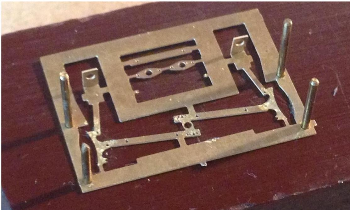
Take the brake shoe infills (14) and fold double with the fold line on the outside.
