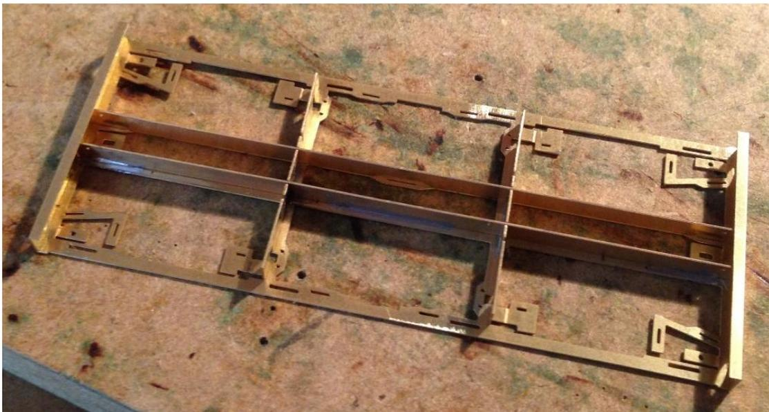
Remove the angled end spacers (4) and clean up any tags. Fit to the underframe using the slots in the transverse spacers and the bottom plate. Solder in place.
