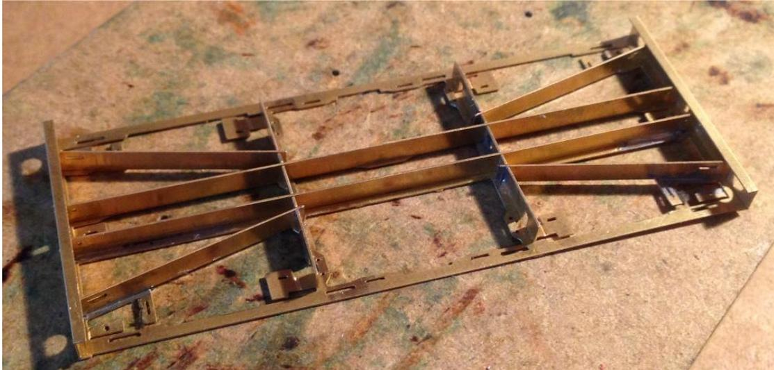
Fold up the buffer and coupling hook guides at the ends of the bottom plate and solder in place.
