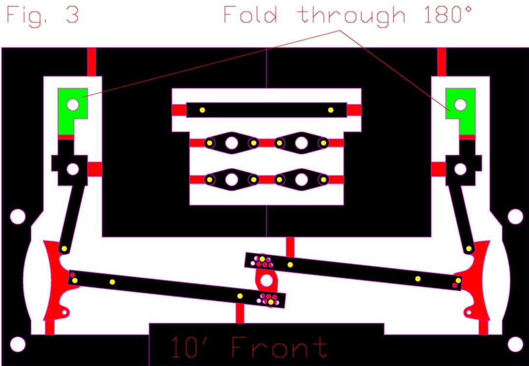
Remove the push rod cranks (15) and push rod infill (16) (if required). Carefully fold the parts marked in green on Fig. 3 through 180°s with the fold line on the outside and then pin to the jig using short lengths of 1mm wire, writing side facing down.
