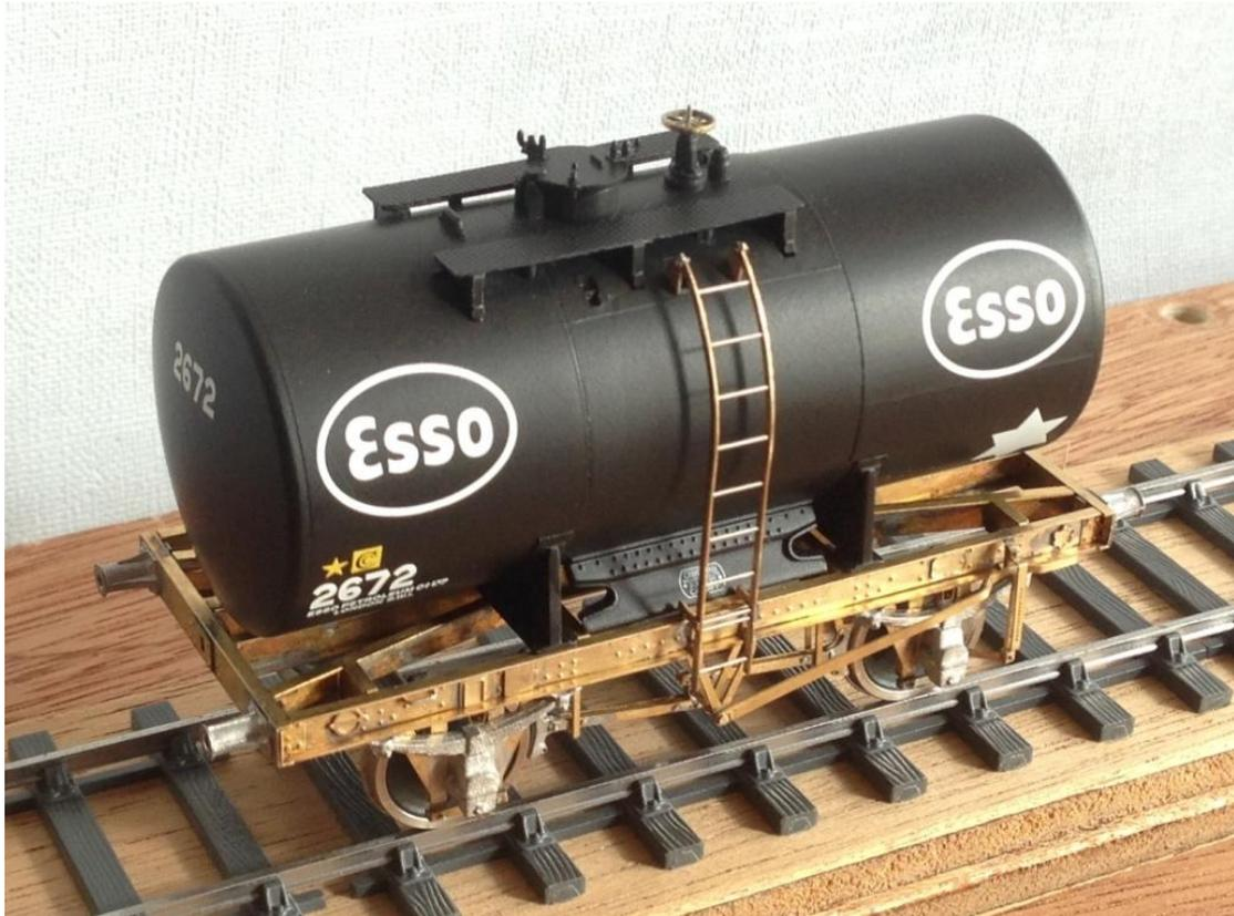
Anchor mounted tanks were introduced in the 1940s and continued to be built into the early 1960s. Indeed I believe that the last unfitted wagon built for use on the British Railways network was an anchor mounted tank wagon built for Berry Wiggins. They were built for various capacities and types of load with different tank diameters. Most common were 14T class A, 14T class B and 20T class B.
