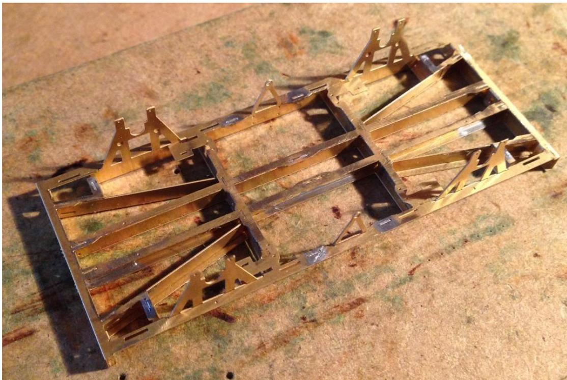
There are four tabs with small slots on into which the brakes will be fitted. Fold these down through 90°s. You should have something that is looking like an open chassis now.
