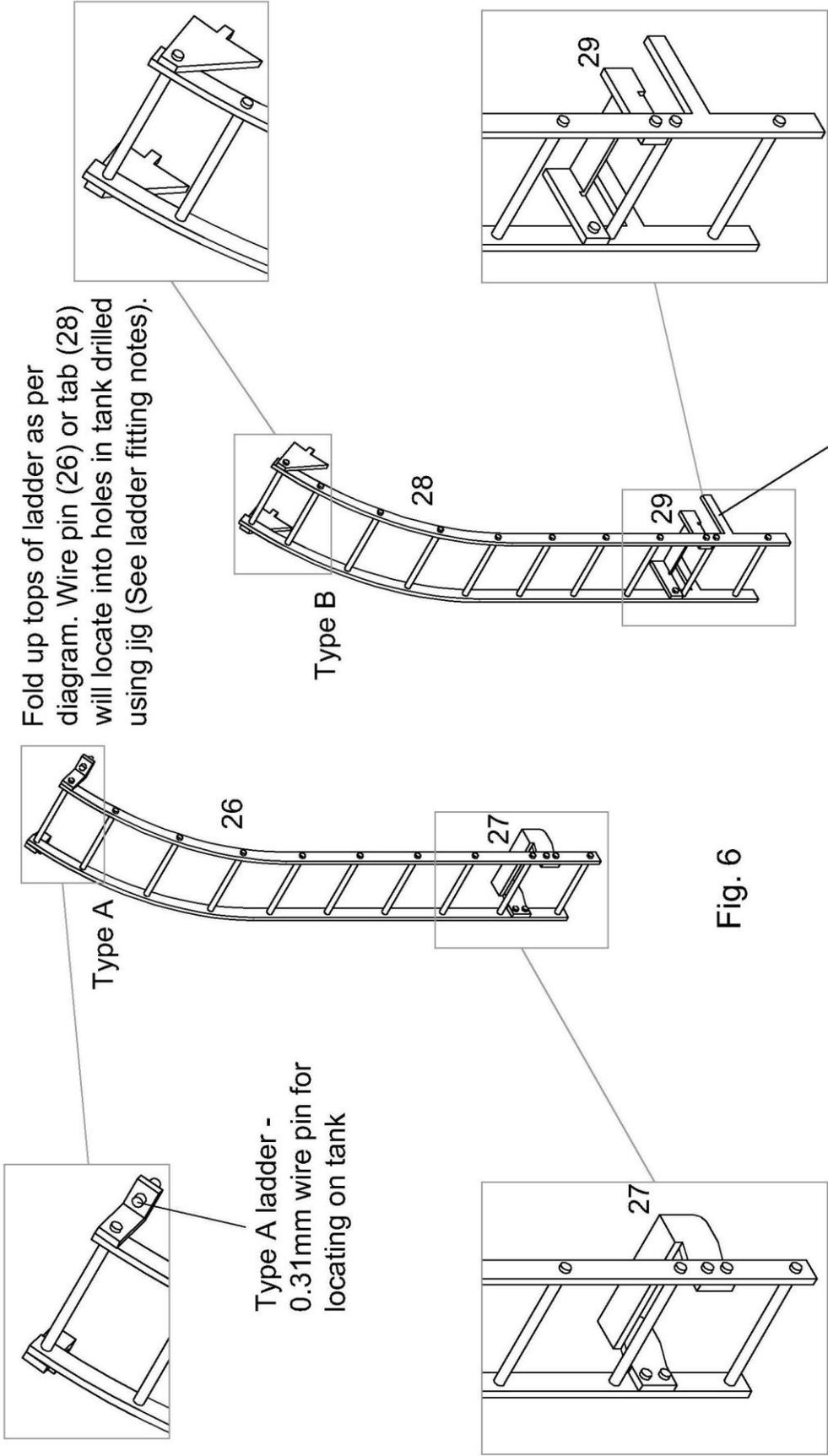
Fold up tops of ladder as per diagram. Wire pin (26) or tab (28) will locate into holes in tank drilled using jig (See ladder fitting notes).
