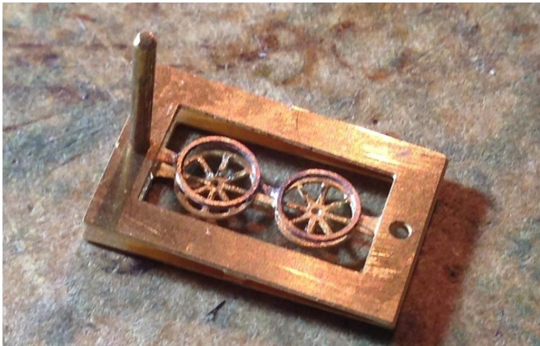
Remove the solid Bachmann valve wheel on top of the tank. To do this make a cut through the shaft immediately below the valve wheel. Carefully drill a 0.4mm hole into the shaft to locate the replacement valve wheel.
