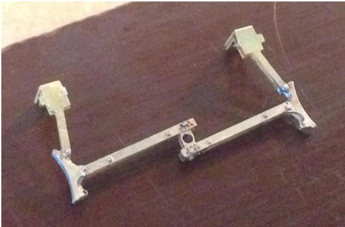
The brakegear can be fitted to the wagon using the tabs and slots as before. Gently bend the shoes to get the tabs into the slots. Use something suitable to pin the brakegear to the chassis through the holes in the feet while you solder them in place.
