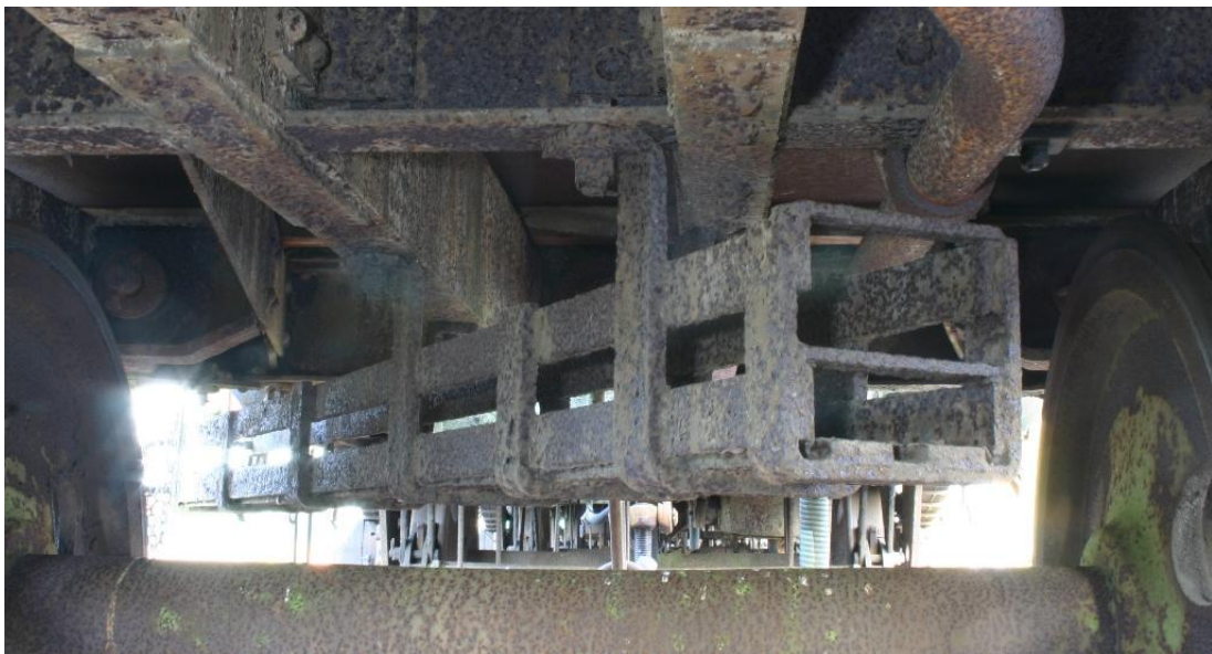
Basket viewed from the inside and showing the basket inner end fill (3)
