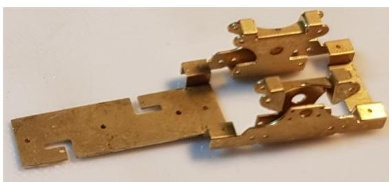
Unlike the photo sequence from here, I would (with hindsight) add the swing link arms next. These are laminated from 3 layers, and it is easier to fit into the frames if the 3 layers are soldered together first – just don't fill the holes (or open them out again).
