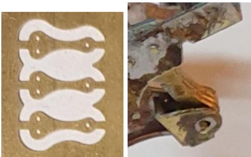
It is also worth adding the the central swing pivot rod at this stage, from 1.5mm OD 1mm ID tube, with a 0.8mm tube and thin rod slightly proud of the end of this – or just a 0.8mm rod inside the 1.5mm tube (see later photos in the sequence, and also the Brassmasters instructions).
