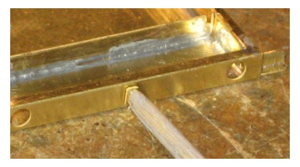
The solebar/Headstock corner plates (15) can also be added. There are two types depending on whether you are making a chassis for a shoc absorbing wagon or not. The type for the shoc absorbing wagons suits the narrower headstock of the prototype. These parts go in the corners between headstock and solebar.
