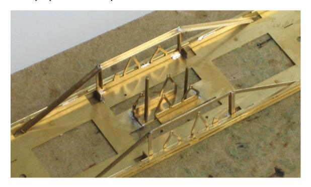
Fix the remaining pieces of brass L section in place at the intersection of truss rods and queen posts.
