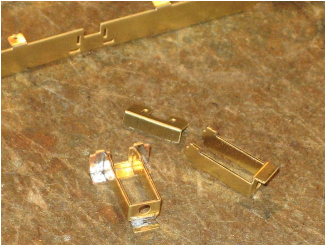
Hymek secondary suspension stirrups and springs.
