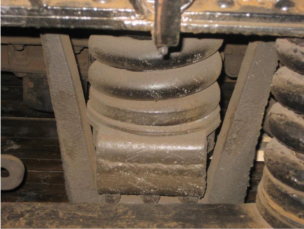
Secondary suspension 'stirrups' and spring seats on an English Electric Type 3. In reality the stirrup is a safety loop and the seat takes the load.
