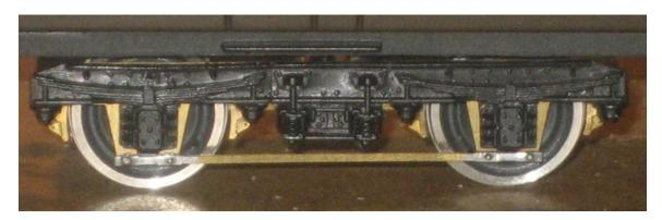
The back of the axleboxes will need to be slotted to allow clearance for the bearings.
