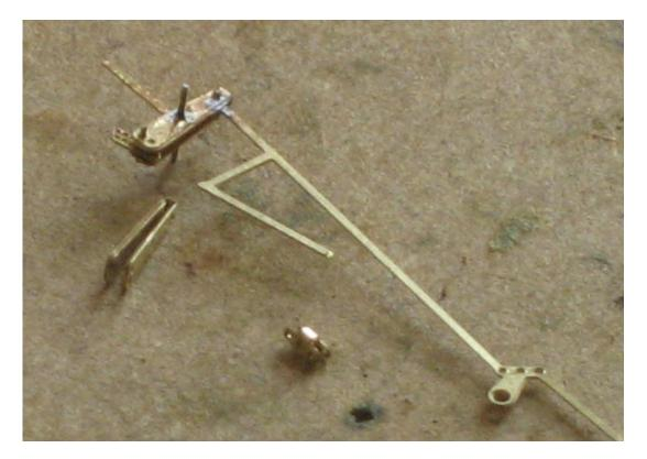
Next attach the brake shaft crank overlays (11) to the centre of the brakegear linkage. Again use 0.4mm wire to attach the overlays and solder in place. The large hole in the centre for the main brake shaft can now be opened out to accept 0.9mm wire.
