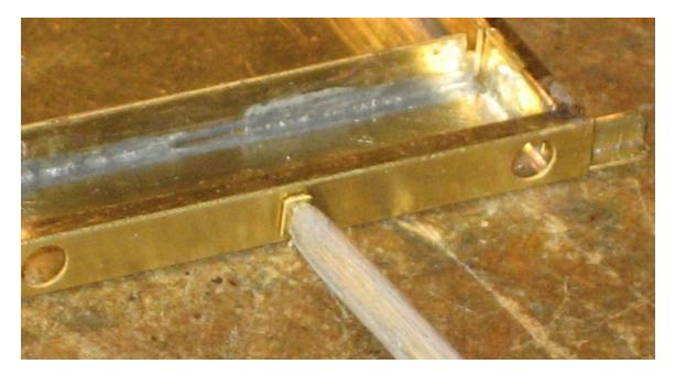
The solebar/Headstock corner plates (15) can also be added. There are two types depending on whether you are making a chassis for a shoc absorbing wagon or not. The type for the shoc absorbing wagons suits the narrower headstock of the prototype. These parts go in the corners below the headstock and solebar.
