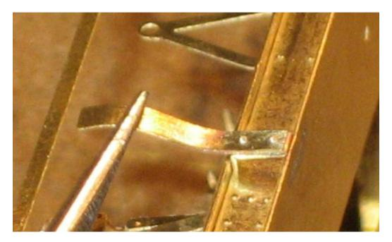
Shocopen wagon door springs (24) are designed to fix behind the solebar for shock absorbing opens. There are locating points on the chassis but note that the springs should coincide with the bang plates on doors which may not be as per the drawing I used to set the locating points. Fold the ends, bend to shape and align appropriately.
