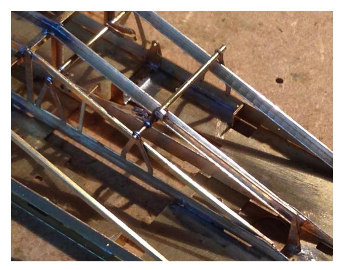
Make sure that the holes in the brake levers (17) and washer attached to them can accept 0.8mm wire and remove from the fret. Fold over the washer and solder in place on the brake lever. Fold up the brake lever so that it clears the solebar (see photo below). Once you are happy with the shape solder in place.
