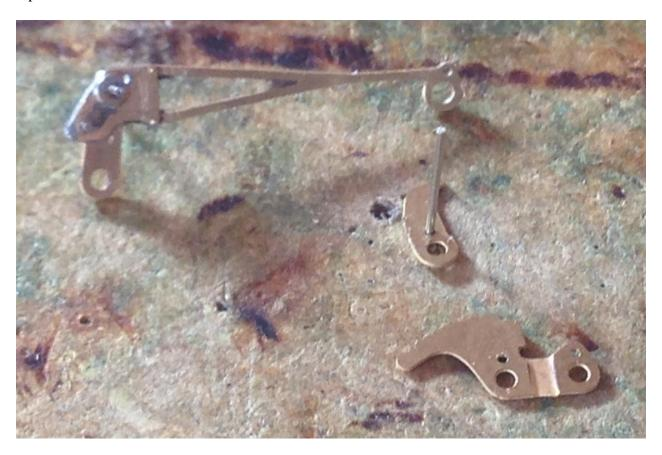
Make sure that the holes in the D/C brake bogie linkage (8) and D/C brake bogie linkage overlays (9) can accept 0.31mm wire and remove from the fret. Attach the overlays by folding around the linkage and then using short lengths of 0.31mm wire to locate them. Solder in place and trim the wire to represent bolt heads. Fold over the locating tab at the end of the linkage.
