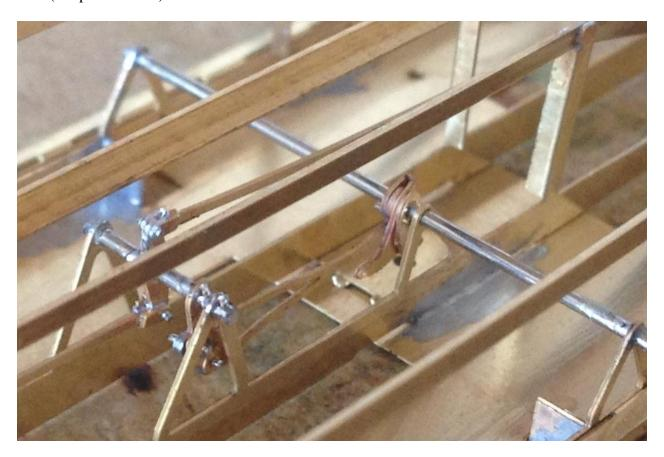
Make sure that the holes in the D/C brake levers (10) will accept 0.7mm wire and fold up. Solder in place on the main brake shaft going across the whole wagon. Note that the position of the brake lever in the photo below indicates that the brakes are on. For the position of the lever with the brakes off, see Fig. 1.
