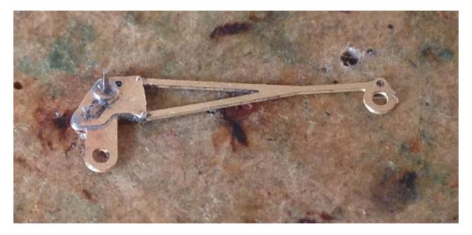
Check that the large holes in the D/C brake ratchet & pawl (8) can accept 0.7mm wire and the small holes 0.3mm wire. These need to be fitted to the brake shaft linkage. Drill a 0.3mm hole in a spare piece of wood and insert a length of 0.31mm wire. Feed the pawl onto the wire as shown in the photo below.
