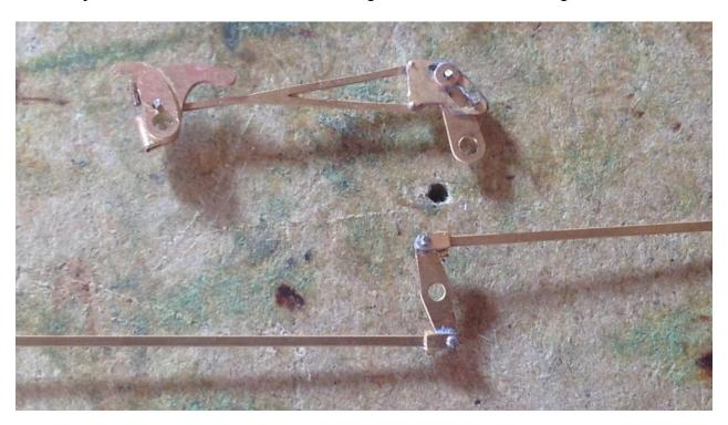
Fit both the brake shaft linkage and bogie linkage to the underframe along with lengths of 0.7mm wire for the brake shafts. Make sure the 0.7mm wire extends 0.5mm or so beyond the vees. The bogie linkage goes along the centre line and the brake shaft linkage goes on the side with the two vees (see photo below).
