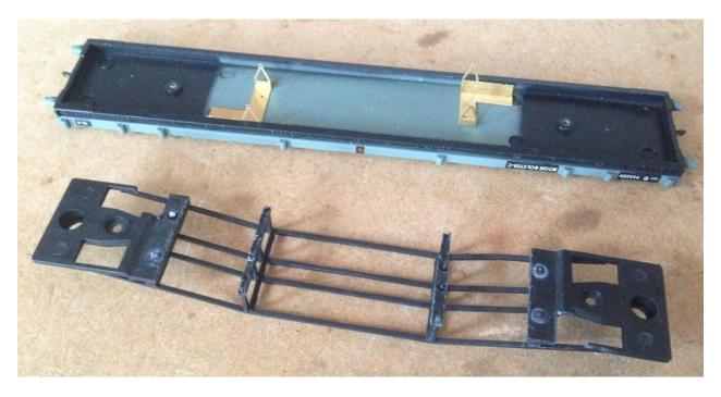
If you are constructing any of the Lever brake options them you will also need to remove a little bit of material from the ends of the trussing where the vees will go. The following photograph will give you a better idea.
