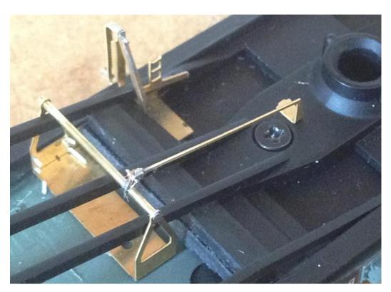
Make sure that the holes in the brake levers (17) and washer attached to them can accept 0.8mm wire and remove from the fret. Fold over the washer and solder in place on the brake lever. Fold up the brake lever so that it clears the solebar (see photo below). Once you are happy with the shape solder in place.
