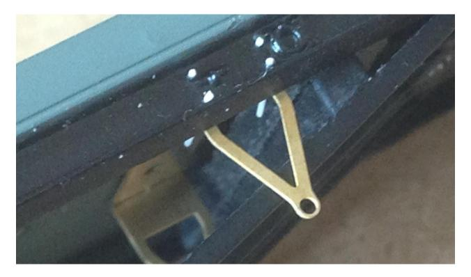
The headstock drilling jig can be folded up and used to drill out holes for buffers and coupling hooks using a 0.6mm drill bit. These can then be opened out to whatever dimension is required. If you are constructing either of the vacuum braked arrangements you can also drill out holes for the lamp irons and vacuum pipe brackets if required.
