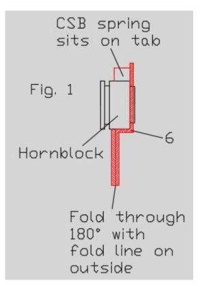
touch with a small file is all that is needed. Thus, the hornblocks/springs should slide freely and smoothly. Fit the wheels, axles and gearbox. Fit the CSB wire through all the holes in the frame spacers and make sure you have a smooth running chassis. Driving wheel washers (8) are provided to take out any side play in the driving wheels but I doubt they will be needed especially in P4.
