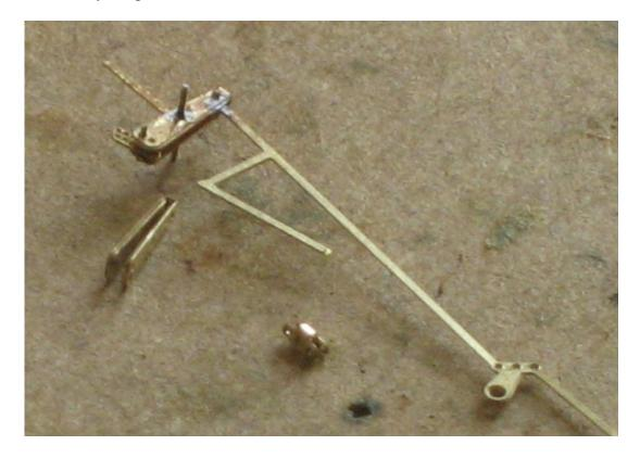
Next attach the brake shaft crank overlays (11) to the centre of the brakegear linkage. Again use 0.31mm wire to attach the overlays and solder in place. The large hole in the centre for the main brake shaft can now be opened out to accept 0.8mm wire.
