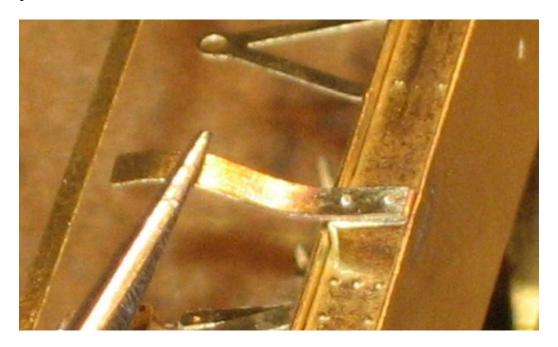
Shocopen wagon door springs (24) are designed to fix behind the solebar for shock absorbing opens. There are locating points on the chassis but note that the springs should coincide with the bang plates on doors which may not be as per the drawing I used to set the locating points. The Parkside Shocopen I have is way out from the drawing in an Illustrated History of BR Wagons Volume 1 which I used as is the Bachmann body. Fold the ends, bend to shape and align appropriately.
