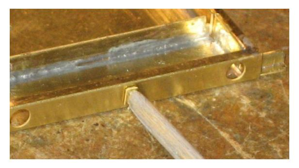
The solebar/Headstock corner plates (15) can also be added. There are two types depending on whether you are making a chassis for a shoc absorbing wagon or not. The type for the shoc absorbing wagons suits the narrower headstock of the prototype. These parts go in the corners between headstock and solebar.
