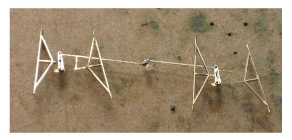
Carefully twist the yolks through 90°s as shown in the photo below.
