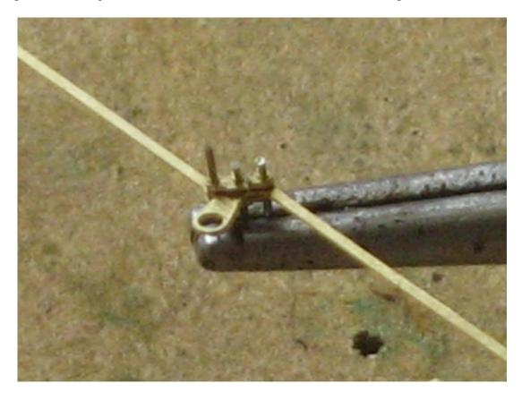
Make sure that there are no half etched connecting tags left on the brakegear linkage (this is important or the yolks wont be in the right place). Fit the yolks to the brakegear linkage using the slots on the yolks and tongues on the linkage. Make sure that they are hard up against each other and solder in place.
