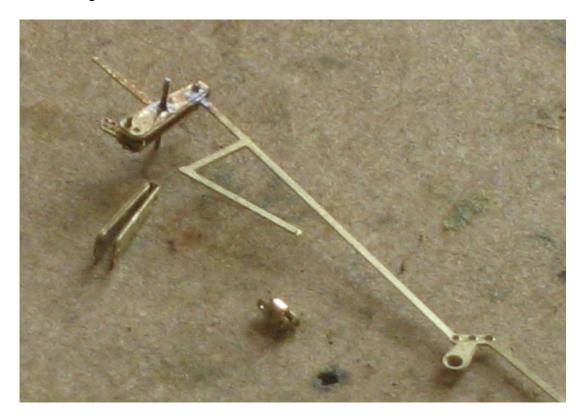
In a similar manner attach the brake shaft crank overlays (10) to the centre of the brakegear linkage. Again use 0.31mm wire to attach the overlays and solder in place. Open out the large hole in the centre for the main brake shaft to accept 0.8mm wire.
