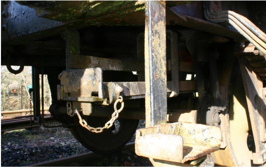
Basket viewed from outer end and showing the basket outer end stop (5)
