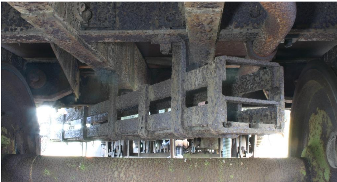
Basket viewed from the inside and showing the basket inner end fill (4)
