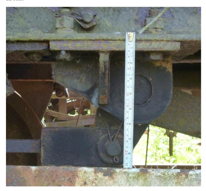
The two vacuum brakegear assemblies can now be fitted to the chassis. Refer again to Fig. 1 for the arrangement. You will need to fit them with a short length of 1.2mm wire for the vacuum cylinder shaft as shown below. Solder the wire to the inner bracket and the vacuum cylinder crank to the shaft at approximately the same position and angle as below. Leave the link free for the moment. Note that the link goes outside of the brakegear and safety loops and inside the axleguard.
