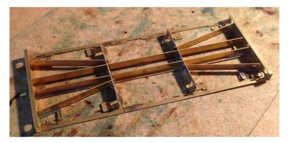
Fold up the buffer and coupling hook guides at the ends of the bottom plate and solder in place.
