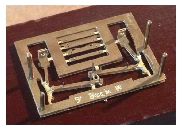
Solder the layers together paying particular attention to the brake shoes (I found it best to apply solder to the long curved edge) and the joints where the wire meet the etch.
