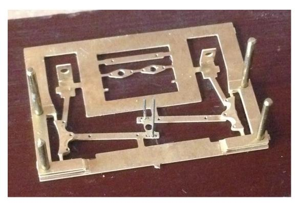
Fold up one set of push rod cranks and place onto the two lengths of 0.31mm wire.
