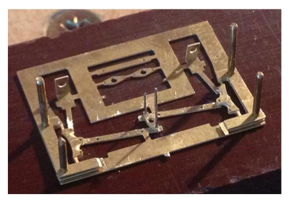
If you wish to use the push rod infill pieces provided then repeat the process for the cranks with theses parts.
