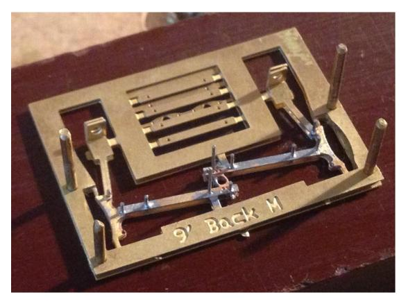
Carefully remove the brakegear from the fret; I used a piercing saw. Clean up any tags that are left and also the wire to represent bolt heads.
