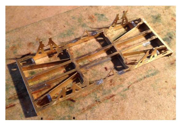
There are four tabs with small slots on into which the brakes will be fitted. Fold these down through 90°s. You should have something that is looking like an open chassis now.
