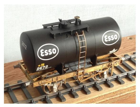
Anchor mounted tanks were introduced in the 1940s and continued to be built into the early 1960s. Indeed I believe that the last unfitted wagon built for use on the British Railways network was an anchor mounted tank wagon built for Berry Wiggins. They were built for various capacities and types of load with different tank diameters. Most common were 14T class A, 14T class B and 20T class B.
