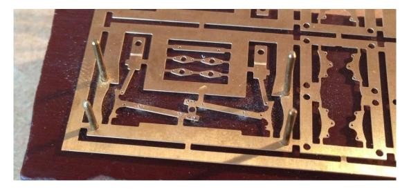
Once the jig is created you can check that the small holes in the rest of the main brakegear (13), brake shoe infill (14), push rod cranks (15) and push rod infills (16) can accept 0.31mm wire. These are marked in yellow on Fig. 3 below. I find it easier to locate the hole from the side with no writing on the main brakegear.
