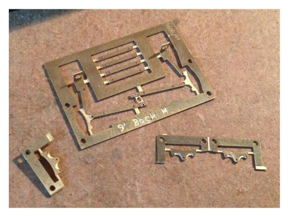
Place the brake shoe infill over the front using the 1mm wire rods to align everything. Insert two short lengths of 0.31mm wire onto the holes where the push rods join the brake shaft cranks.
