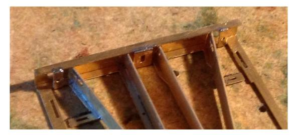
Check that the large holes in the vees on the top plate (5) will accept 0.8mm wire and the small holes for the secondary vee pins and horse hooks can accept 0.31mm wire. Drill out the holes on the backs of the axleguards as per your particular prototype (they did vary and some didn't have any) using a 0.85mm drill then remove from the fret.
