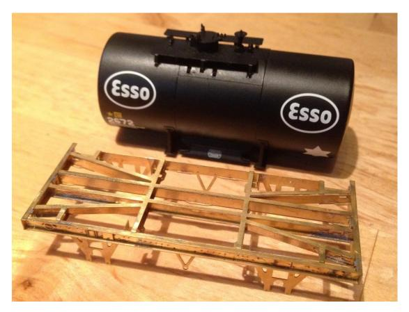
The solebars can now be fitted to the chassis. There are slots and tabs on the bottom plate to aid location and the ends go into the channel that is the headstock. Fit the solebars at an angle and then straighten, locating the slots and tabs at the same time. Once in place then the solebar can be soldered in place.
