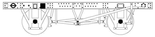
**B.73** BR Plate axleguards used on later 15-20T wagons, principally bitumen tanks.
