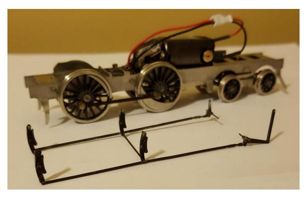
The test chassis was built with 0.5mm ID tube in the frames, and wire stubs in the breakgear assembly, so that it can be clipped on and off as required for maintenance, painting, etc. This is something you may want to consider doing.
