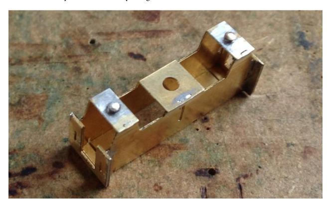
The brakegear detail (5) comes as a simple fold double part. Remove from the fret and fold about the middle so that the fold is through 180° with the fold line on the outside. Use the part to drill a pair of 0.3mm holes into an off cut of wood or mdf. Insert two short lengths of 0.31mm wire into the holes and through the brakegear detail. Solder the wire in place and the two halves of the brakegear detail together. Trim the wire to resemble bolts.
