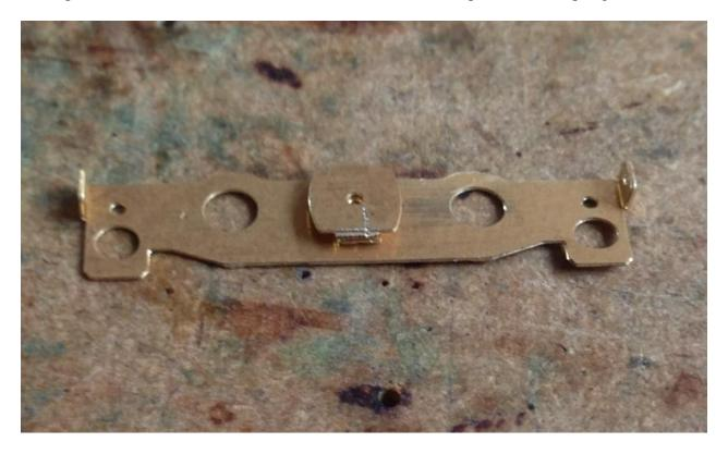
At this point use the sideframe to create a jig using a piece of scrap wood or mdf onto which everything can be placed. This will mean drilling two 2mm diameter holes where the bearings will go, a 0.7mm hole through the cam and two 0.7mm holes just above the bearing holes. Use two short lengths of 2mm diameter rod to keep align things in the bearing holes.
