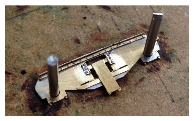
Remove the lower angle flange (10) and solder in place using the slots and tabs to locate.
