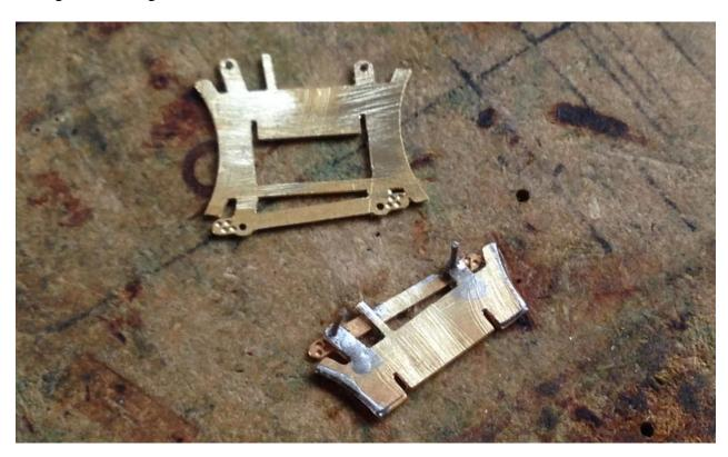
Insert the brakegear detail into the slots on the underneath of the bolster. The two sets of brakegear detail for each bogie form a mirrored pair and should be arranged the thin push rod going between the two brake shoes is towards the outside of the bolster.
