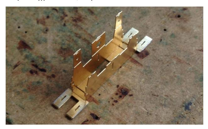
Then fold the ends up so that the slots engage with the tabs on the bolster sides. Solder the sides to the sides from the outside corner. Make sure the parts are hard up against each other and only use a little solder so you avoid getting any on the inside face of the ends between the bolster sides.
