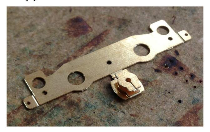
As mentioned before the functional part of the sideframes consists of a cam that fits into the slots in the sides of the bolster. The cam consists of three parts, two smaller and one larger which need to be folded up. Start with the fold line furthest from the main part of the side and fold through 180° with the fold line on the outside. Repeat for the next fold line. You will end up with the arrangement illustrated in the previous picture.
