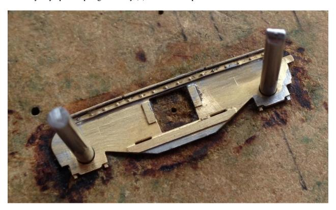
Next remove the bolster guide overlay (9) from the fret. Note that the bar connecting the two little detail parts should be retained until the overlays are soldered in place (see photo below). Use the connecting bar to locate the two overlays and solder in place. You can then use something like a small scalpel or chisel blade to cut the connecting tags.
