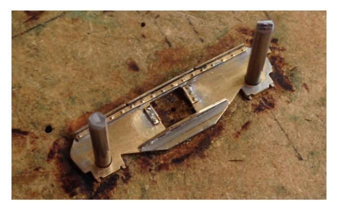
Carefully tidy up the lower angle overlay (11) and solder in place.
