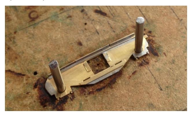
Carefully tidy up the top angle overlay (8) and solder in place.
