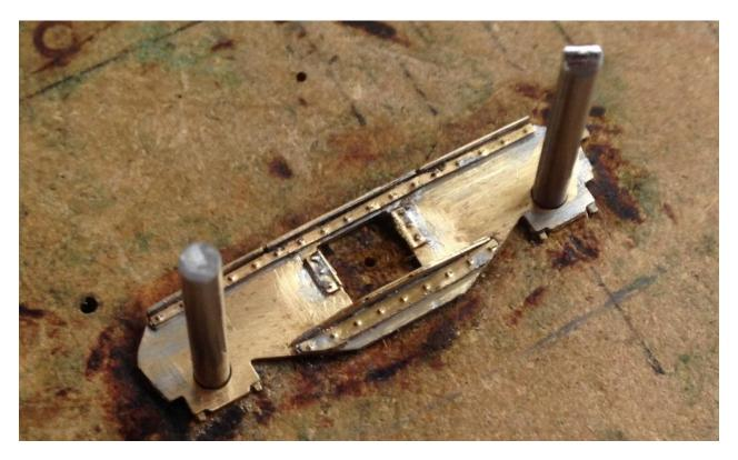
Dress the edges of the flanges on the top and lower angles with a file and remove form the jig.
