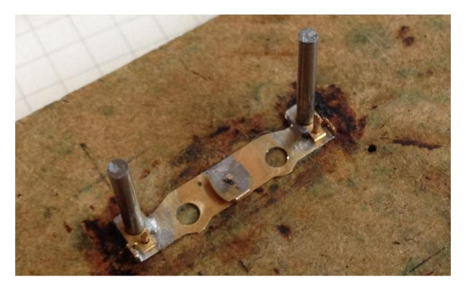
Trim the lace pins so that it is flush with the sideframe on both sides.
