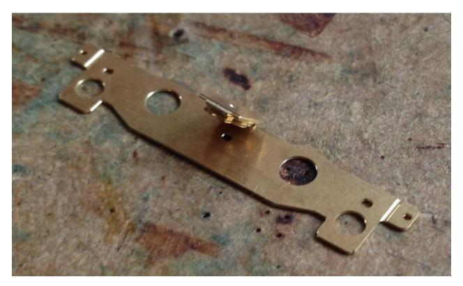
Fold up the two tabs at the ends which will become the fulcrum points for the spring wire.
