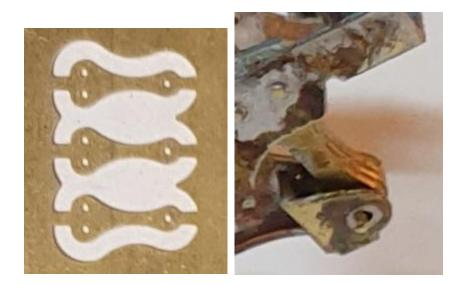
It is also worth adding the the central swing pivot rod at this stage, from 1.5mm OD 1mm ID tube, with a 0.8mm tube and thin rod slightly proud of the end of this – or just a 0.8mm rod inside the 1.5mm tube (see later photos in the sequence, and also the Brassmasters instructions).
