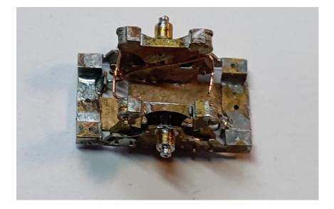
As per the Brassmasters instructions, presuming the coil spring method is being used rather than hornblocks – thickening strips need adding to the axle guides. When these are folded up and the hornguides are added, the top of the horns are wider on the inner face and need filing back to be flush with the sides of the spring guides (this step will only be required if using the spring attachment points).
