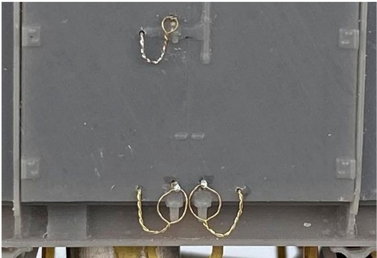
BR 'New Build' fitted - Lower chains fixed to body, no padlock, door clasp pin in place with chain and secured to the end of the door clasp. Wagon modelled empty.
