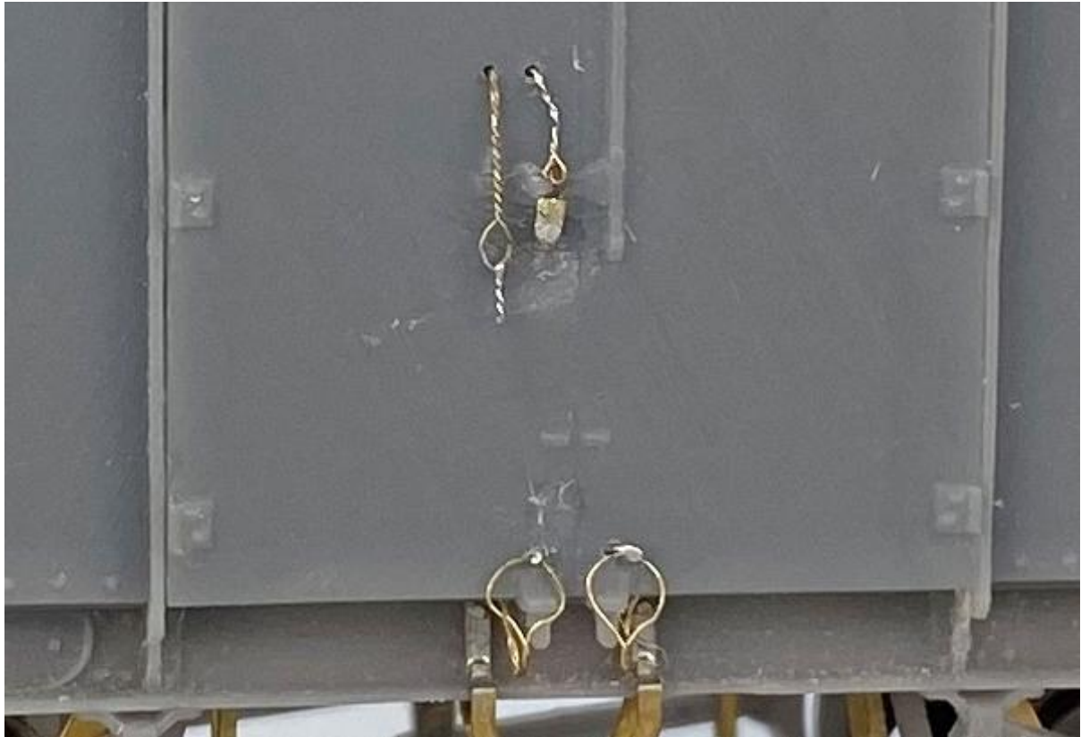
LMS Unfitted - Lower chains fixed under body, padlock on chain and secured from above, representation of clasp pin hanging on chain.
