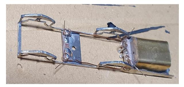
There is a little depth on the keeper spacers to locate pcb for attaching pickups to. You can get very thin PCB sheet from Eileen's Emporium. It's listed under their miscellaneous section. I fitted pickups to the spacer for the front driving wheels and to the front of the ashpan for the rear driving wheels, each on a PCB strip.
