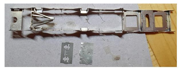
For the Craftsman build I fitted the slidebars first, then cut them to clear the hornguides. On this build I fitted the hornguides first, and then cut the slidebars before fitting them butting up to the hornguides. I think the former was easier, but the latter ended up looking neater as the cut was easier to do and clean up when as a separate piece on the workbench. Fitting it and aligning it was tricky as it wasn't then pre-jigged at both ends.
