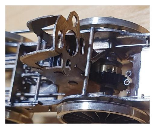
This gearbox is pushing the limits of the space, but it fits well in the round topped firebox version but does need the top corners of the gearbox rounding off to follow the curve of the motor.
