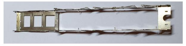
2 - Remove the appropriate set of frame spacers (3(i), 3(ii), 4, 5 & 6) from the fret. The spacers for EM are the b set. Those for P4 are the c set. Fold up spacer 6 into a C shape. See Fig 1. If fitting slidebars (8) you must fold them up and fit to spacer 3 before fitting to the chassis. Note that the
