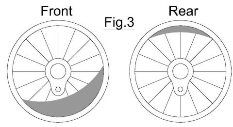
If you haven't fitted the balance weights (32) then do so now. They should be arranged as follows. The front wheel is shown as per the left hand side. The right hand side should be a mirror of this.
