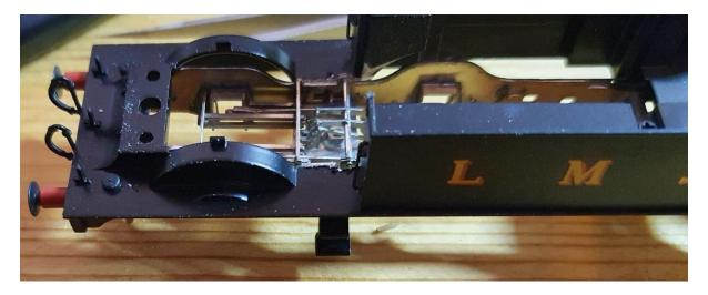
I added a roll of 1.6mm lead sheet into the boiler, and 3 sheets in the tanks. There is room for more if required in the ashpan and bunker, but these options don't put it in an ideal location for adhesion. Check the fit of the 3D printed boiler bottom. This can be painted before fitting if you want.
