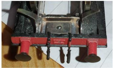
Remove and fold up the rear body fixing bracket (36). The part is designed to concertina together and both fold lines are through 180° with the fold lines on the outside. The 3 middle holes should be used to align the bracket with the rear of the chassis where it sits on top of it.
