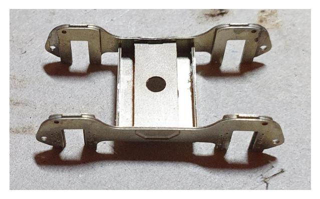
Fold up bogie bolster (28b or c) and add its frame spacer (28d). The eight short fold lines around the central rectangle with the hole in are through 90°, the other four are through 180° with the fold line on the outside. Solder together with 0.5mm wire through the holes in the cosmetic 'compensating beams' to resemble bolts.
