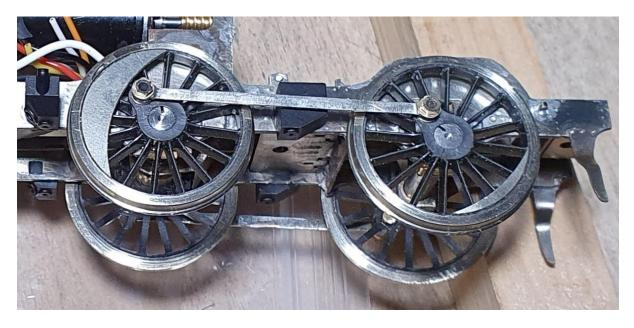
As can be seen in the above photo, the axles on the test build were slotted with a piercing saw. This was to help allow the wheels to be pinned. The slot was used as a guide for a small drill through the wheel centre, and then glue a piece of wire in once happy with quartering and running qualities. This isnt completely necessary, but a belt and braces option.
