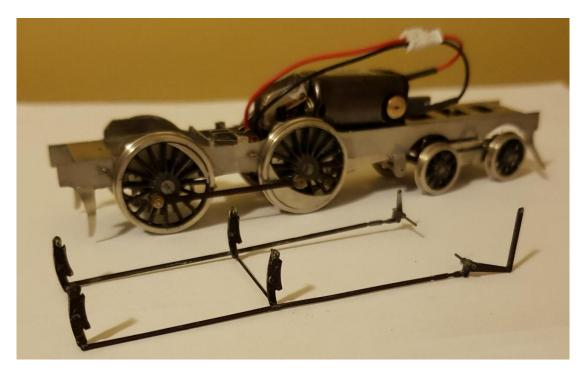
11 - Fit a brake shaft made from 1mm wire, or tube along with appropriate steam brake crank (23) (various positions and can be fitted to either side - check your prototype) and hand brake crank and link (24). The latter fits to the LHS. Folds the part double with the fold line on the outside and use 0.5mm wire to represent a rivet.
