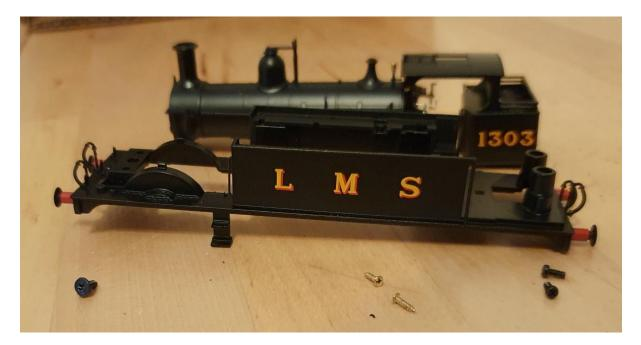
The splashers will need opening out to clear the wheels. Use a slitting disc in a minidrill/Dremel. The footplate also needs filing back behind the splashers to allow the frames to fit between them.
