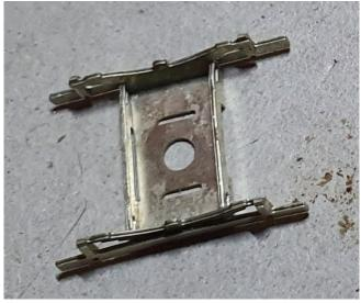
To assemble the bogie, make two long L shaped springs from the smaller spring wire approximately 26mm x 1.5mm. Fit hornblocks to bogie frame making sure they are in the correct place. Place the bolster on top of bogie. Fit spring wire through hornblock then bolster then hornblock on the other axle. Fit short tail of spring into hole on bogie frame mentioned earlier to retain the spring wire and stop the bogie coming apart.
