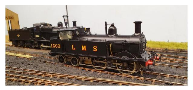
The chassis was originally developed to suit the Craftsman kit, which is still available (Rumney Models X.04A), and while most of the build follows the same concept, the chassis has been reworked to suit the Bachmann body. 3D printed components such as sandboxes and a brake cylinder are included so that these items do not need to be removed from the Bachmann chassis. A printed boiler bottom is also included to fill the gap left by the removal of the Bachmann mechanism.
