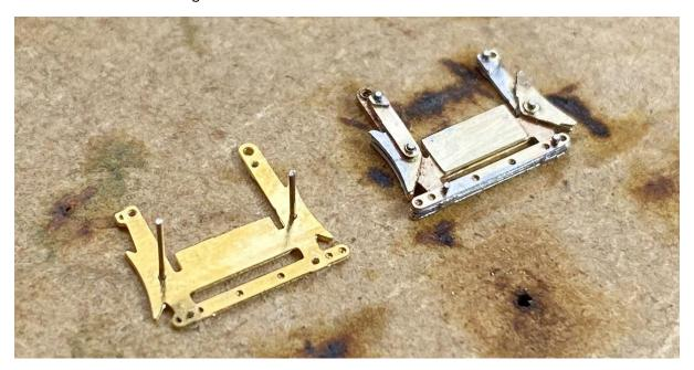
Place the front main layer (4b) on top of the back part using the two wires to align things. Insert 4 short lengths of 0.31mm wire into the remaining holes shaded yellow in Fig. 1 above and which you have already opened out.
