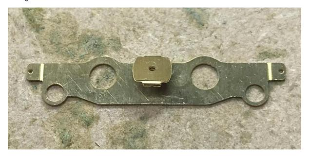
Use the sideframe to drill a 0.7mm hole into a scrap piece of wood or mdf. Insert a length of the lace pin shank through the cam and into this jig. Solder the cam in place making sure the various parts are hard up against each other. Again, use only the minimum of solder and try and keep it from spreading along the sideframe (a paste flux maybe useful here).
