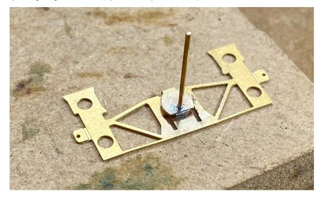
Fold the two parts that will represent the back flange of the journal through 180° with the fold line on the outside. Solder in place.
