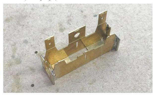
Fold over the three top parts so the tabs and slots engage, and solder in place. Solder the lace pins in place and then cut the shank of the pins so that only a little remains beneath the top. Retain the shank of the lace pins as this will be put to good use later.
