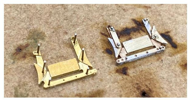
Next, add the pull rod detail (4c) and the brake shoe/hanger detail (4d). Note that part 4d goes on the side with the larger hole at the top of one of the hangers.
