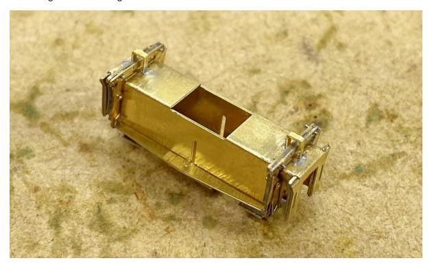
Remove the brakegear safety loops (4h) from the fret and fold into a C shape. Insert into slots in the bottom of the bolster and solder in place. See above image.
