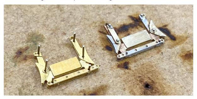
Finally, add the brake shoe detail (4e) to the opposite side to part 4d and the brake hanger detail (4f) on top of part 4d so everything looks like the set of parts on the right in the image above.
