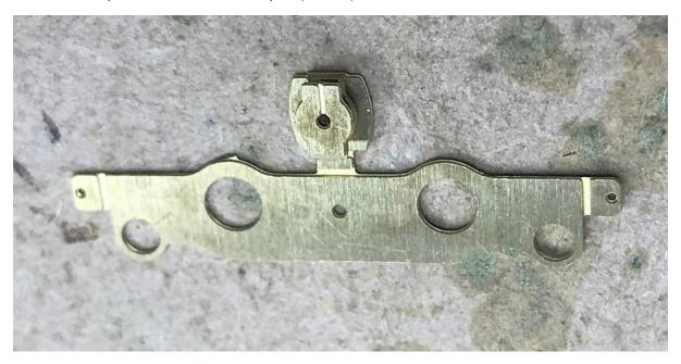
As mentioned before the functional part of the sideframes consists of a cam that fits into the slots in the sides of the bolster. The cam consists of three parts, two smaller and one larger which need to be folded up. Start with the fold line furthest from the main part of the side and fold through 180° with the fold line on the outside. Repeat for the next fold line. This will produce a sort of concertina effect. You will end up with the arrangement illustrated in the previous picture.
