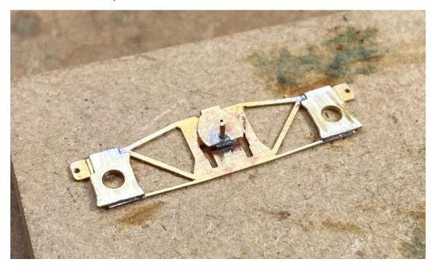
Fold up the two tabs at the ends which will become the fulcrum points for the spring wire and reinforce with solder.
