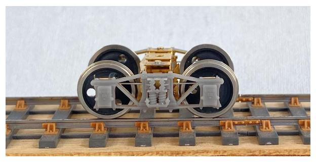
The bogies are designed to be built with sideframes that are sprung to the bolster. These are held in place by the spring wire, and they can be easily disassembled for easy removal of the wheels should the need arise. You will need 2mm top hat bearings to complete along with your choice of 3'1" wheels. Note that waisted type bearings are not suitable for these bogies as the cosmetic 3D printed parts of the sideframes rely on the bearing to align them.
