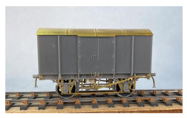
The kits are a mixed media affair, mainly in 3D printed resin but with a sprung brass 'under frame', roof (for a prototypically thin look) and detailing parts along with a cast whitemetal vacuum cylinder (where appropriate). You will need wheels/bearings, buffer heads, coupling links (hooks and Instanters are provided) or screw couplings (Rumney Models B.96 for these) and some ingenuity/material for the door chains along with paint and transfers. The padlocks now come printed in place.
